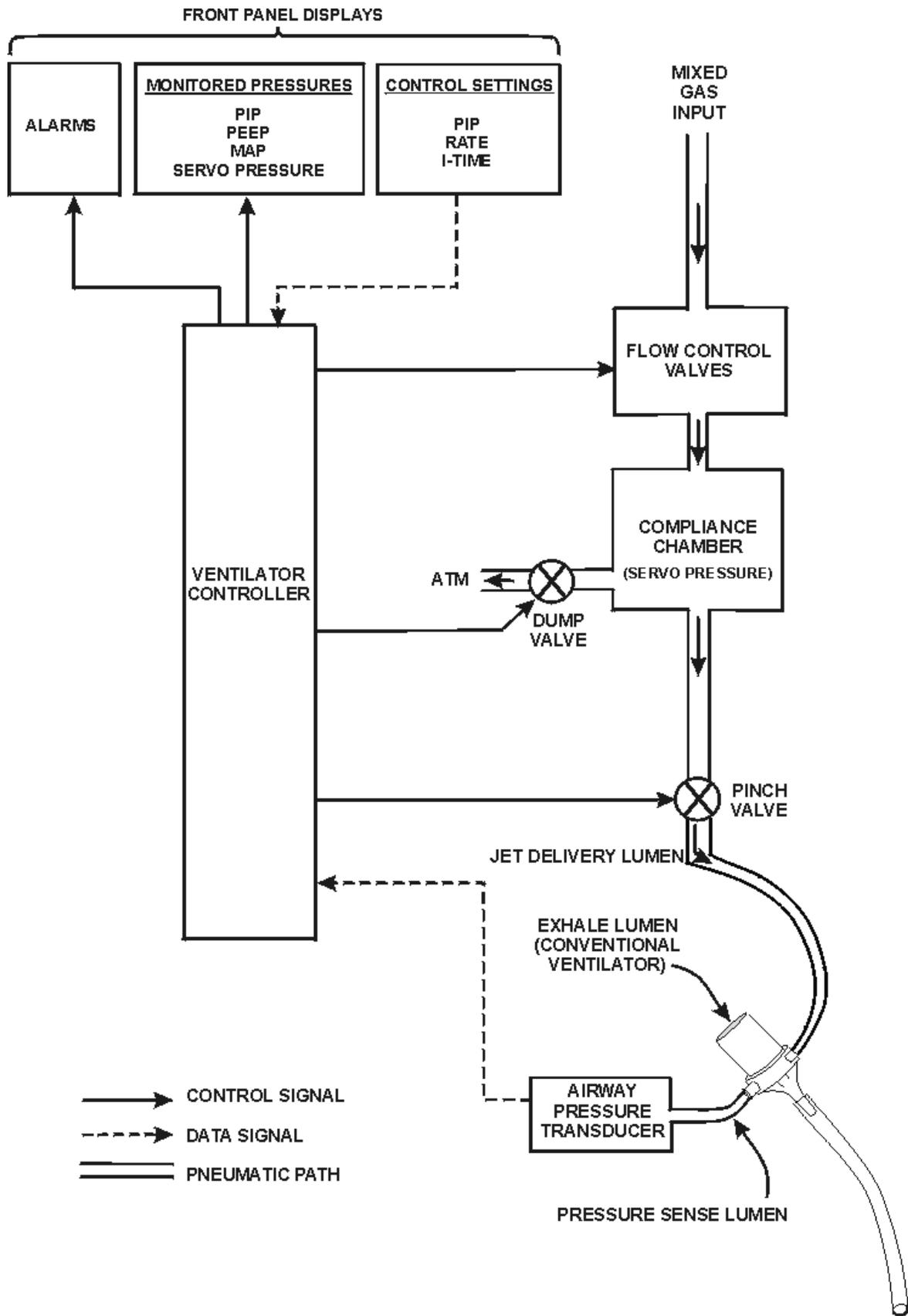
Figure 3: Feedback Control of PIP Using "Servo Pressure"
