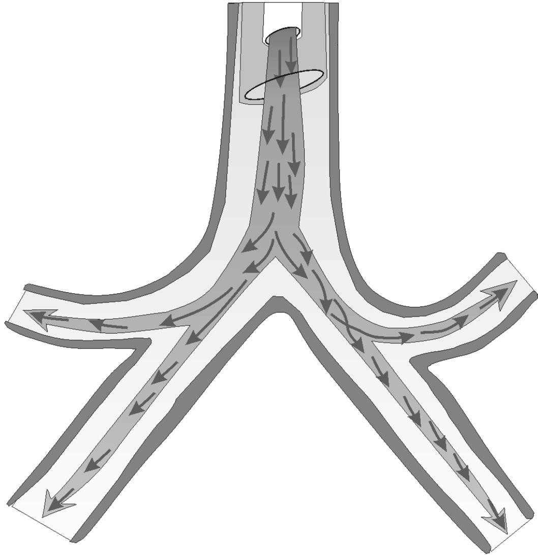
Figure 5: The Jet squirts gas into the lungs as fast as possible. The inspired gas penetrates down the center core of the airways where resistance to flow is lowest, leaving considerable CO<sub>2</sub> in the airways at end-inspiration. *Effective* dead-space volume is thereby reduced since only portions of the anatomic dead space are used.
