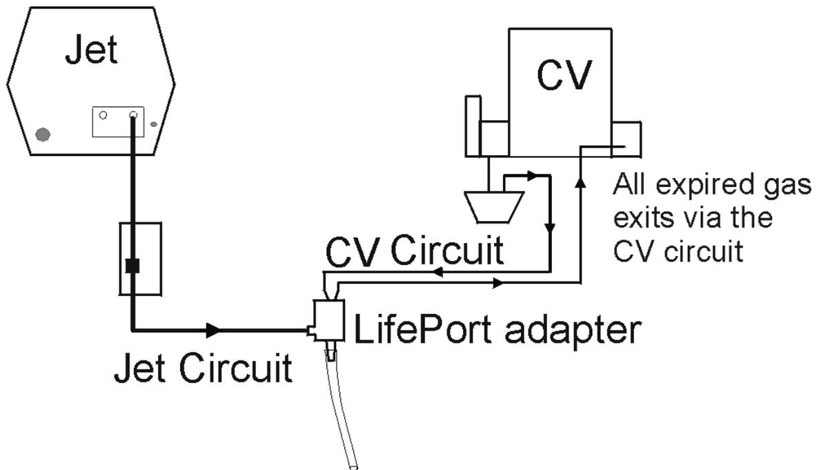
Figure 4: A conventional ventilator is always used in parallel with the Jet. It provides gas for the patient's spontaneous breathing, and it delivers occasional "sigh" breaths to recruit collapsed alveoli if atelectasis is present.
