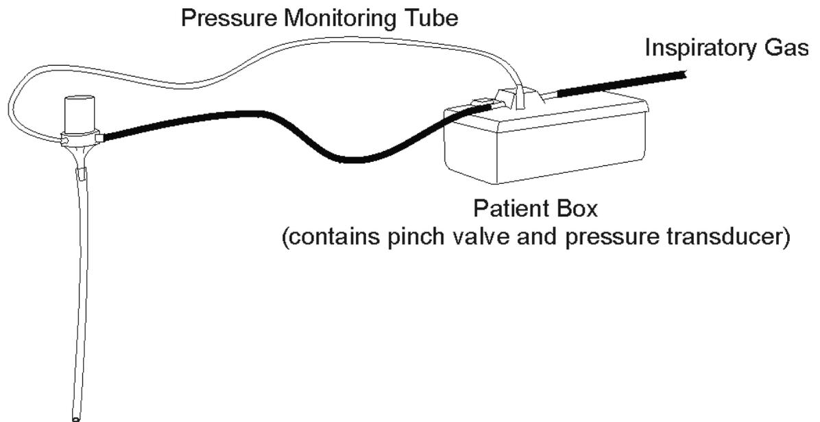
Figure 2: "Patient Box" Delivers HFJV and Monitors Airway Pressure
