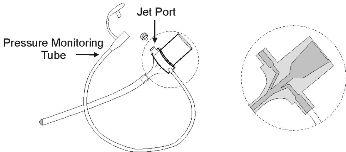
Figure 1: LifePort Endotracheal Tube Adapter
