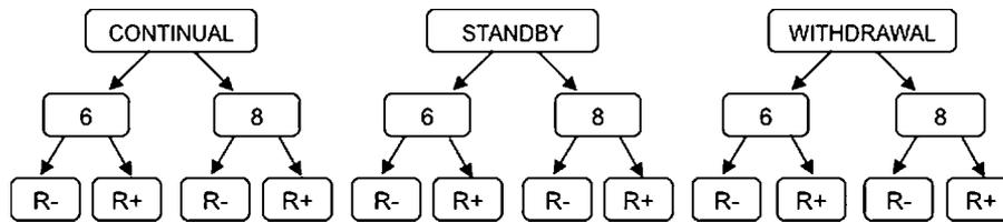
Fig. 1. Summary of the 12 suction permutations performed randomly in each subject (four different permutations for each method of suction, *Continual*, *Standby*, and *Withdrawal*). 6: 6FG catheter, 8: 8FG catheter, R-; represents episodes performed with no recruitment, R+; represents episodes performed with post-suction sigh inflations (3 BPM).
